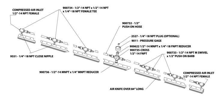
Pipe thread sealant should be applied to all threads (small packet included). Avoid the inside diameter of the fitting so it does not enter into the Air Knife.
