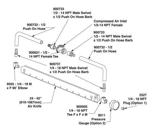
Pipe thread sealant should be applied to all threads (small packet included). Avoid the inside diameter of the fitting so it does not enter into the Air Knife.
