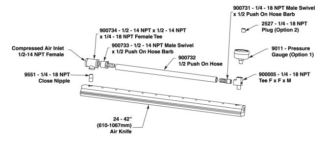
Pipe thread sealant should be applied to all threads (small packet included). Avoid the inside diameter of the fitting so it does not enter into the Air Knife.
