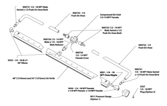
Pipe thread sealant should be applied to all threads (small packet included). Avoid the inside diameter of the fitting so it does not enter into the Air Knife.
