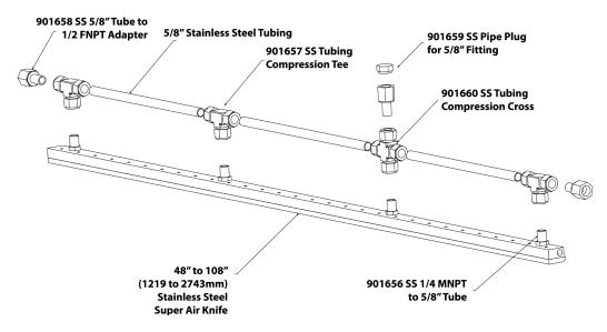
Pipe thread sealant should be applied to 901656 inlet threads (small packet included). Avoid getting the sealant on the inside diameter of the fitting so it does not enter into the Super Air Knife.
