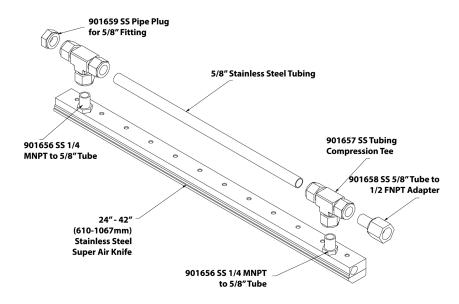
Pipe thread sealant should be applied to 901656 inlet threads (small packet included). Avoid getting the sealant on the inside diameter of the fitting so it does not enter into the Super Air Knife.
