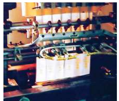
A Model 2012 12" (305mm) Standard Air Knife opens mustard packets prior to fill.
