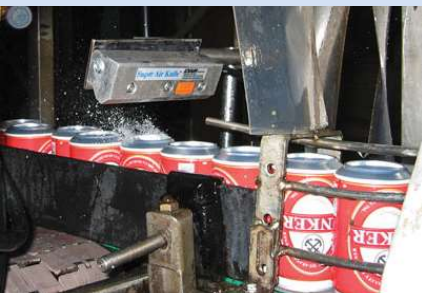
Model 110006 6" (152mm) Super Air Knife removes residual water from can bottoms after a rinse process, eliminating water damage to packaging and shipping materials.
