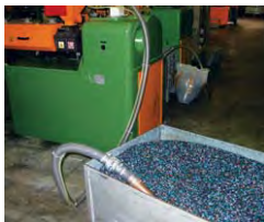
The Model 6083 1-1/2" (38mm) Line Vac conveys plastic granules to the gravity feed hopper on an extruder.
