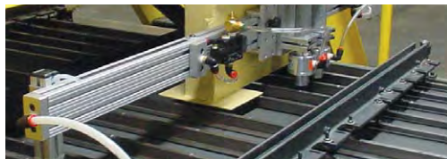
(2) Model 6083 1-1/2" (38mm) Line Vacs convey rejected metal caps from a fluorescent lamp operation to a scrap bin.
