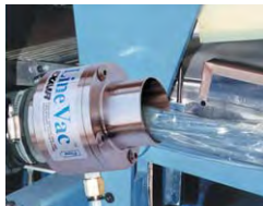
A Model 6084 2" (51mm) Line Vac transports scrap cellophane trim to a waste barrel.
