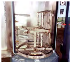
(3) Model 2012 12" (305mm) Standard Air Knives perform the drying cycle in this parts washer.
