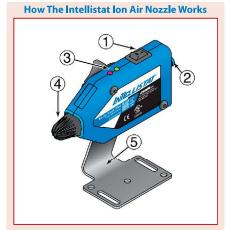
After connecting the 24V power supply, activate the power switch (1) and turn on a compressed source to supply the 6mm push-in fitting (2) to activate the static eliminating ions and airflow. Proper or improper functionality is indicated by a green or red LED (3). The non-marring nozzle (4) provides  $\ quiet performance \ and \ OSHA \ compliance. \ The \ compact$ mounting bracket (5) is included to provide handsfree operation.
