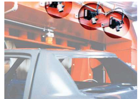
(3) Gen4 Ion Air Cannons blow contaminants from car bodies prior to painting.
