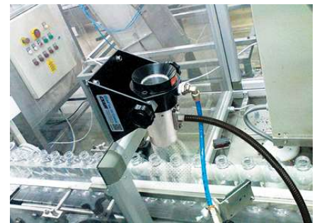
The Model 8292 Gen4 Ion Air Cannon System eliminates the static and dust prior to filling the bottles.
