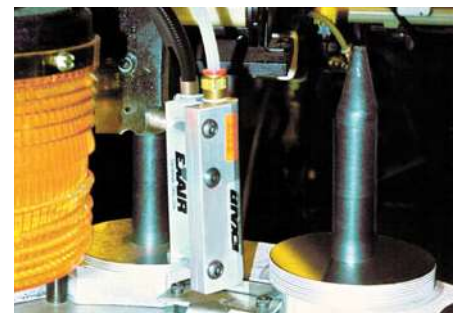
A Model 8103 3" (76mm) Gen4 Standard Ion Air Knife removes dust from computer hard disks prior to assembly.
