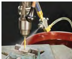
A Model SR10105S is used to supply a cooling mist for a drilling operation.
