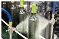
(2) Model EB10305S atomizing nozzles are used to give a final sanitary rinse prior to labeling wine bottles.
