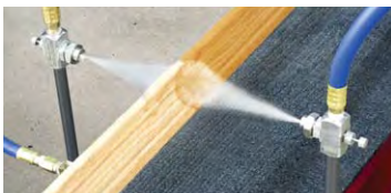
(2) Model ER1020SS atomizing nozzles are used to apply a fire retardant coating to wood trim.
