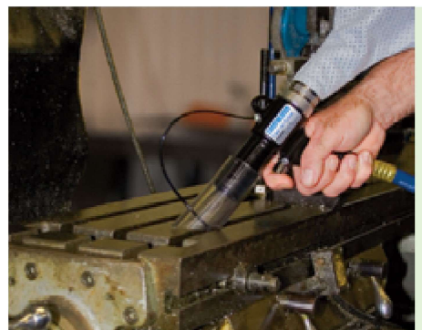
The Model 6194 Deep Hole Vac-u-Gun cleans the t-slots on a milling machine.
