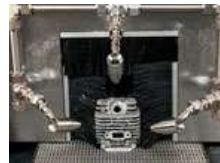
A combination of Model 6013 High Velocity Air Jets dry this chainsaw cylinder head.
