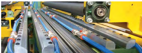
A series of Full-Flow Air Knives "float" layers of plastic film in the confined space of the machine.
